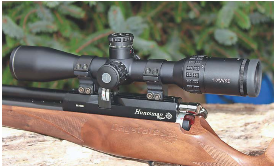
The Regal needed high mounts to clear the magazine.
