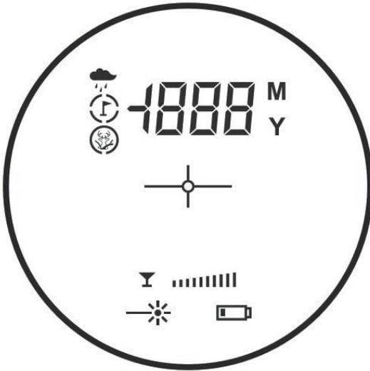
**LRF reticle has all you need to start successful rangefinding.**
