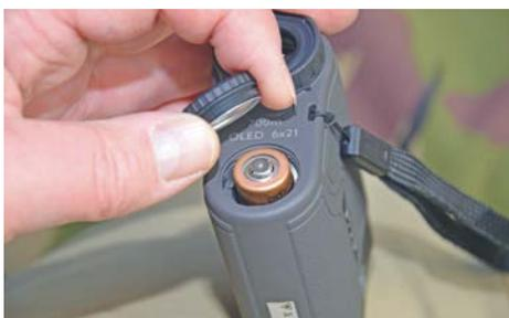
The battery cover simply screws off to expose the CR2 battery
