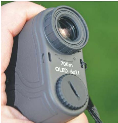
Note the dioptre adjuster at the top and the slots on either side for the wrist strap
