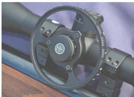
With the side wheel in place, note the distance markings
