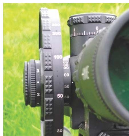
I would have liked a simple parallax pointer provided with the wheel, to give a more visible indexing mark than the tiny white dot on the turret base
