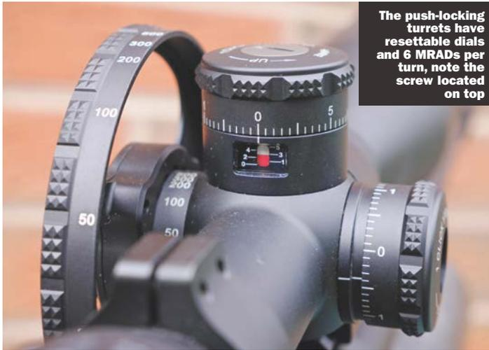
The push-locking turrets have resettable dials and 6 MRADs per turn, note the screw located on top
