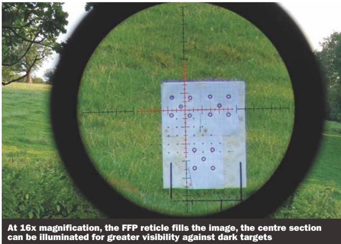
At 16x magnification, the FFP reticle fills the image, the centre section can be illuminated for greater visibility against dark targets
