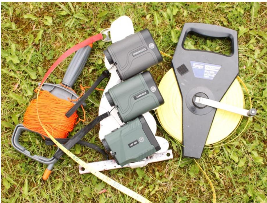
I tested the 55-yard measurements with a tape and metal knock-down FT target.
